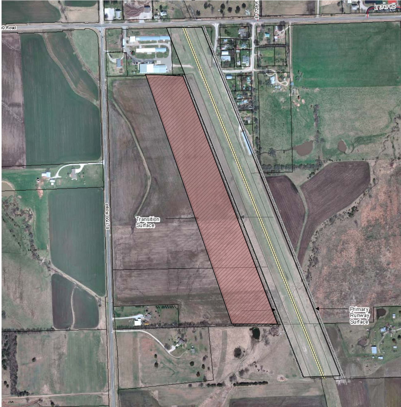
Primary Runway Surface And Transitional Surface Figure 2
