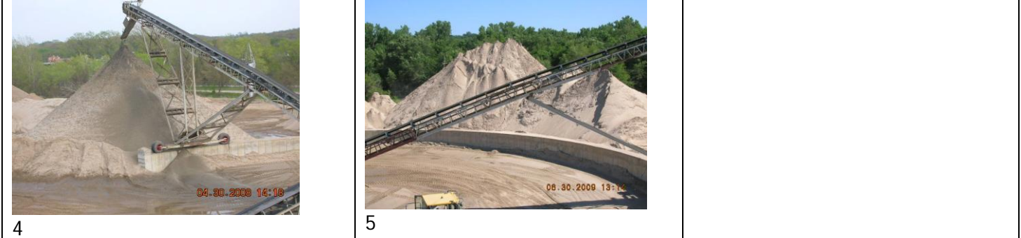
Samples of stockpiling. Radial stacker piling finished product. Conveyors up to 50' tall.
