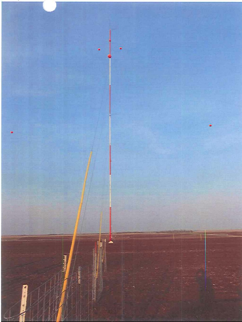
Winch/bridle anchors can be seen in photo (above left) – 45 feet from mast center, no guy wires, marked with t-posts and hi-visibility guy sleeves. Outermost-anchor – 164 feet from mast.
